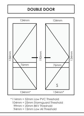
The stable door displacements are based on standard 72mm Outer Frame all round
