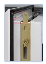
To adjust the shootbolt throw 10 to 13 mm, move the mushroom cam so that the plastic pin locates into the desired position. This should be done before either cropping the extension to size, or locating the extension into the rapid-fix drive gear.
