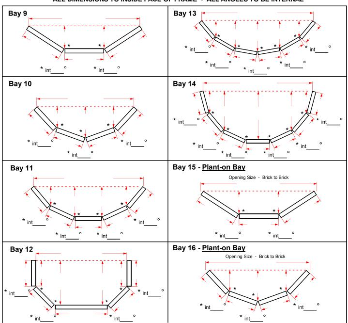
Note: Please ensure that all information and <a href="INTERNAL DIMENSIONS">INTERNAL DIMENSIONS</a> are provided, this will ensure orders are processed without delay. Details of the Windows/Doors that go with this bay plan must be entered on our official order form. Load bearing bays will be supplied with pole jacks.
