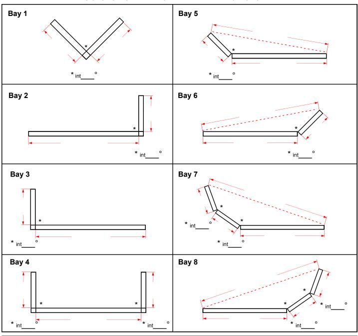
Note: Please ensure that all information and <u>INTERNAL DIMENSIONS</u> are provided, this will ensure orders are processed without delay. Details of the Windows/Doors that go with this bay plan must be entered on our official order form. Load bearing bays will be supplied with pole jacks.
