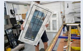
Climatec's R7 products are manufactured with three joint options. You can choose the fully mechanical option with glass bonded units, opt for sashes with our ETL welds or just go for a fully welded product.
