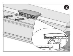
Fasten the sash plate with screws M 3,9 x 38 mm.
