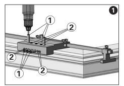
Fix the jig in the right position. Drill in correspondence of bushes 1 with a drill bit Ø 7,2 mm and in correspondence bushes 2 with a drill bit Ø 3,0 mm.
