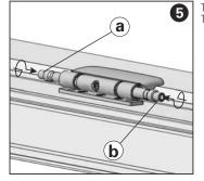
Twist in pin **a** flush fit to the upper ring. Twist in pin **b** till it touches the central rin
