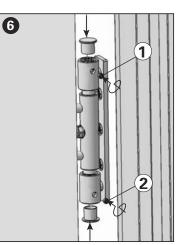
Fit the caps and fasten the security screws 1 and 2
