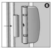
Unscrew the security screws and remove the caps
