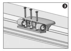
Fasten the frame plate with fastener 3,9 x 38 n **IMPORTANT:** trim the of the rings towards the plate.
