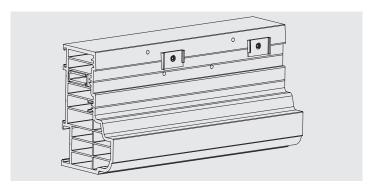
Fit the two frame spacers on the outer holes.
