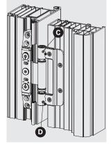
Insert the sash into the frame and screw in the pin with a 4mm Allen Key until the measure 6mm is reached. Open the sash and screw in the security screws marked and .
