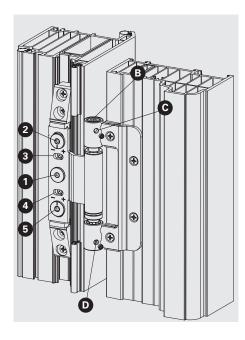
Horizontal adjustment: unscrew by three turns, screw 1. Tighten or loosen alternately screws 3 and 4 with a 4mm Allen key. Tighten screw 1. Adjustment ±3mm.
