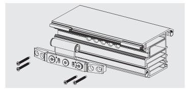
Fasten the sash part into the eurogroove with fasteners suitable for the material of your door
