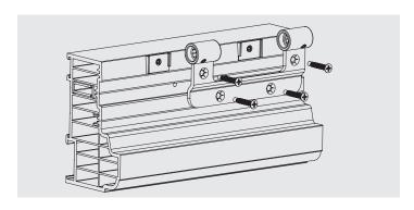
Fasten the frame plate with suitable fasteners for your door
