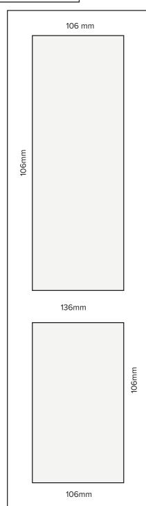
The door & coupled side panel displacements are based on standard 72mm outer frame all round, 107mm midrail and 69mm transom for window. Dimension of coupler for door should be added.
