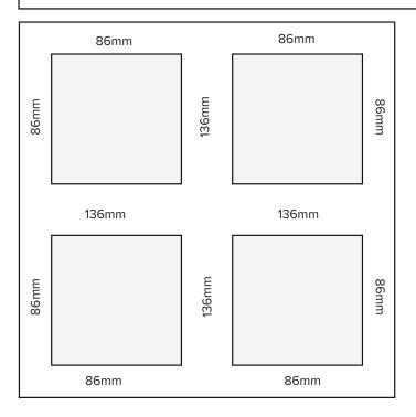
The Flush Casement Window displacements are based on standard 52mm outer frame and 69mm transom and mullions. If using 62mm outer frame, add 10mm to the dimensions around the perimeter. If using 72mm outer frame add 20mm.
