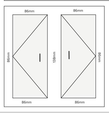
The double hung displacements are based on 52mm outer frame and 69mm floating mullions. If using 62mm outer frame, add 10mm to the dimensions around the perimeter. If using 72mm outer frame add 20mm.
