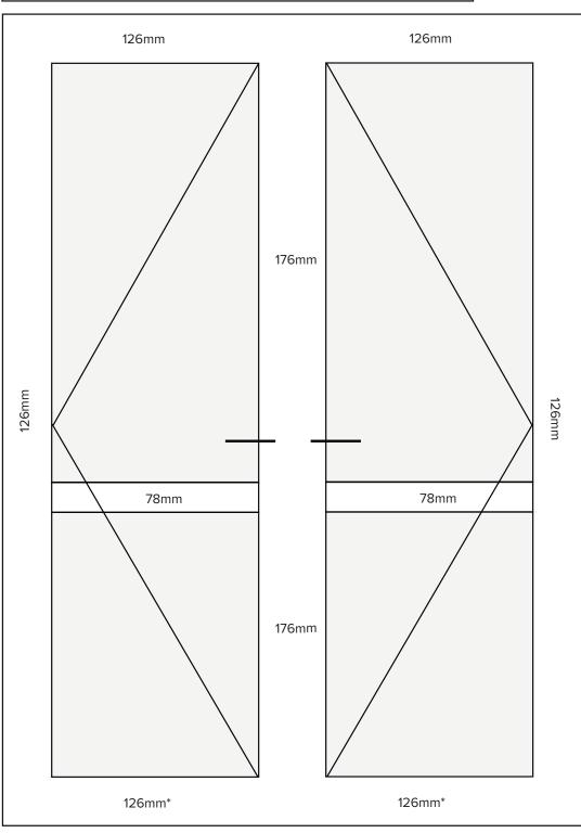
The double door displacements are based on standard 72mm outer frame all round & 107mm midrails.
