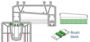
Run silicone along the inside of cill upstand, position against the frame and screw together at 300mm centres.
