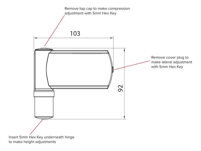
Adjustment is carried out in three directions with a standard 5mm Allen key.
