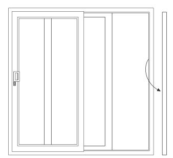
3. The vertical cover profile can then be removed to allow for fixing.
