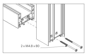
Screw the frame profiles together and then tighten the loose screw connection of the vertical frame profile.
