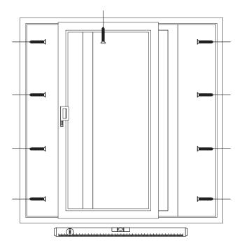
4. Fix the door using appropriate fixings. Corner fixings should be between 150mm and 250mm from the external corner. Intermediate fixings should be at centres no greater than 600mm. Screws should be fixed into the brickwork, not the mortar.
