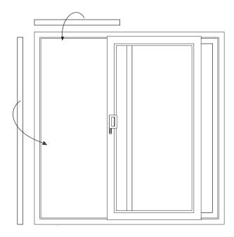
7. Re-insert the cover profiles into the sliding sash side starting with the horizontals first
