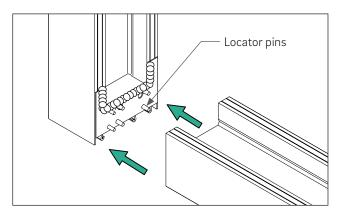
Connect horizontal and vertical frame profiles to each other. The "locator pins" help to place the frames in the correct position.
