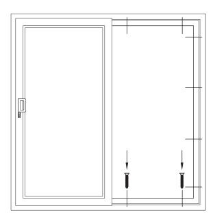
5. Re-clip the trims into the fixed side frame, slide the fixed sash back into position and secure with the fixing screws.
