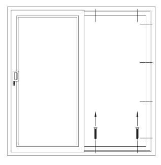
1. Remove the cover profiles from the sliding sash side, starting with the aluminium tread plate. It may be necessary to remove the handle and bump stops to enable the door to slide far enough back for easier removal.
