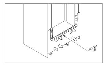
Before screwing the vertical frame profile to the horizontal, seal with silicone as shown in the illustration.
