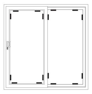
6. Glaze the doors, starting with the outside sash. Pack the glass accordingly. The bottom bridge packers should be placed above the position of the rollers. This is approximately 150mm from the corners.
